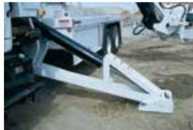
Extension stabilizer cylinders are designed to withstand the rigors of changing off-the-road tires. The cylinders are fully protected to provide longer component life and reduce maintenance.
