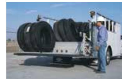
IMT electric-hydraulic liftgates feature a unique hydraulic cylinder lift design that reduces the downtime experienced with cable-lift models. Corrosion-resistant nonskid grated platforms provide secure footing and long-lasting visibility of your company's identification package. Integrated lighting, power shutoff safety switch, tire-stop and siderail are standard.
